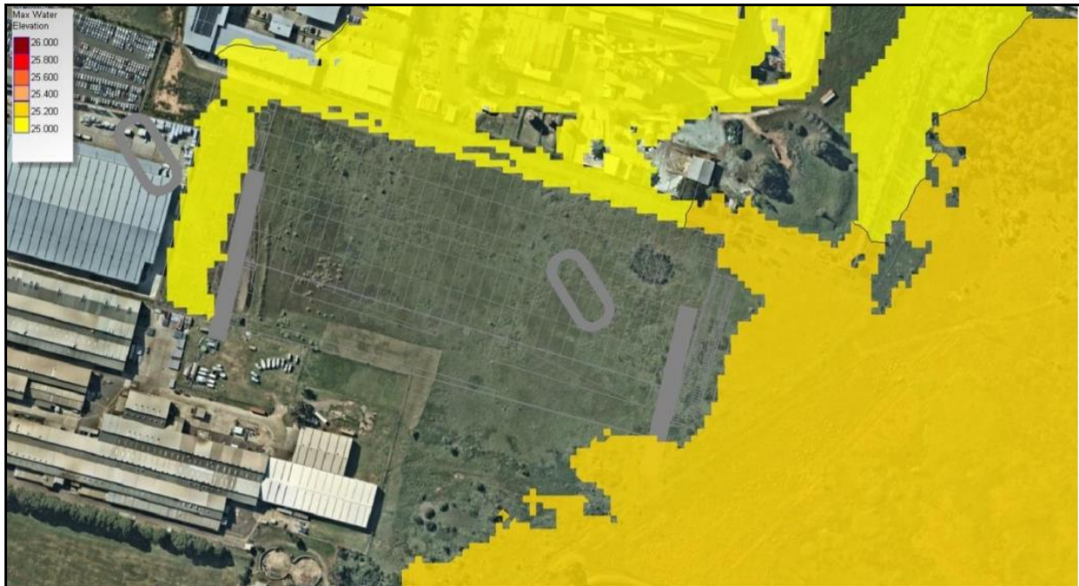
Figure F8 – 1% AEP Flood Levels – Post Development
