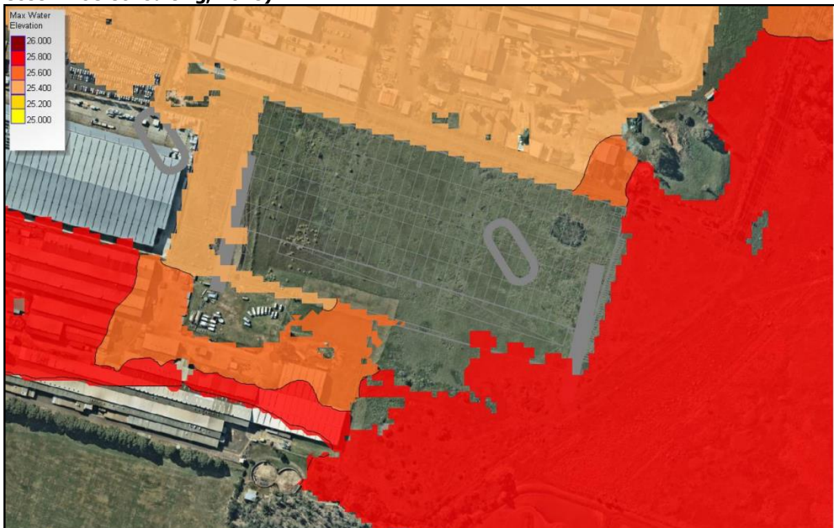
Figure F14 – 0.5% AEP Flood Level – Post Development
