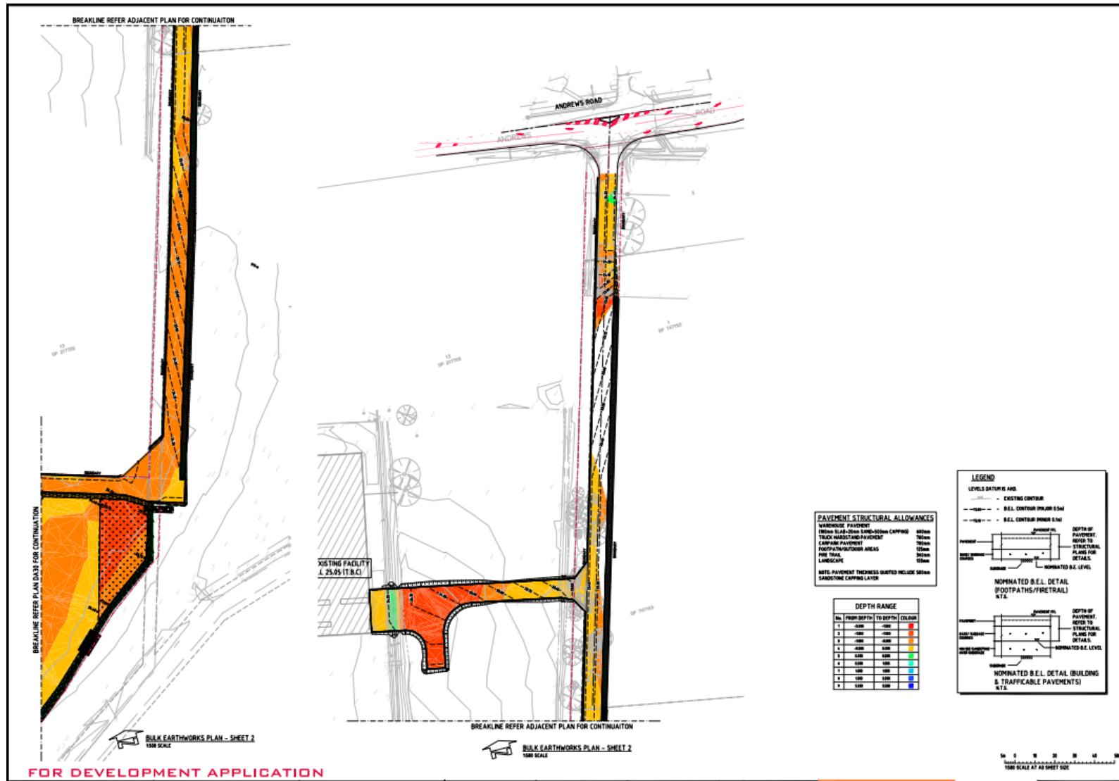
Figure 16 Proposed Bulk Earthworks at the Subject Site Access Road (Source: Costin Roe Consulting, 2018)
